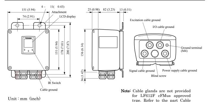
Figure 5. Separate type converter LF612 and LF612F
