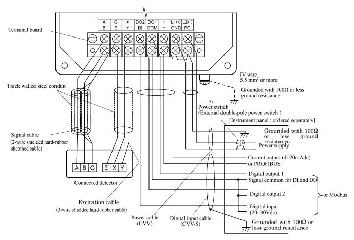
Figure 7. Separate GF632/LF612 and GF632/LF612F type Converter Wiring Diagram
